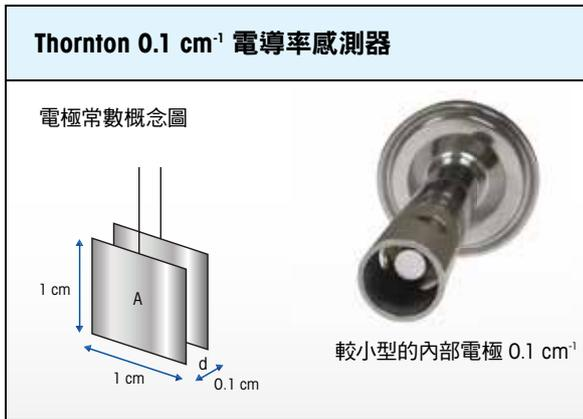
$$\text{電導率電極常數} = \frac{\text{長度}}{\text{面積}} = \frac{0.1 \text{ cm}}{1 \text{ cm}^2} = 0.1 \text{ cm}^{-1}$$
